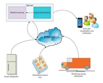
Fig. 2. The implementation scheme of mobile e-nose for beef quality monitoring
