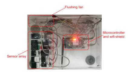
Fig. 3. The prototype of MoLen sensor box
