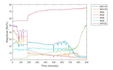
Fig. 4. E-nose signals during beef spoilage process
